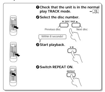
• The disc number can be selected directly by using the **DISC SELECTOR** and numeric keys in place of the **DISC SKIP** keys.
